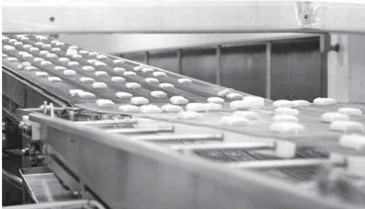
Dough travels by conveyor on Mama Rosa's newest mini pizza production line that makes 500 pizzas a minute.
