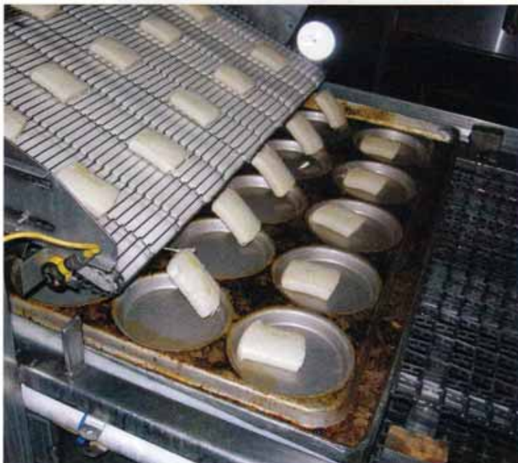
▲ Dough pieces are conveyed into pans on bakery line No. 3.
