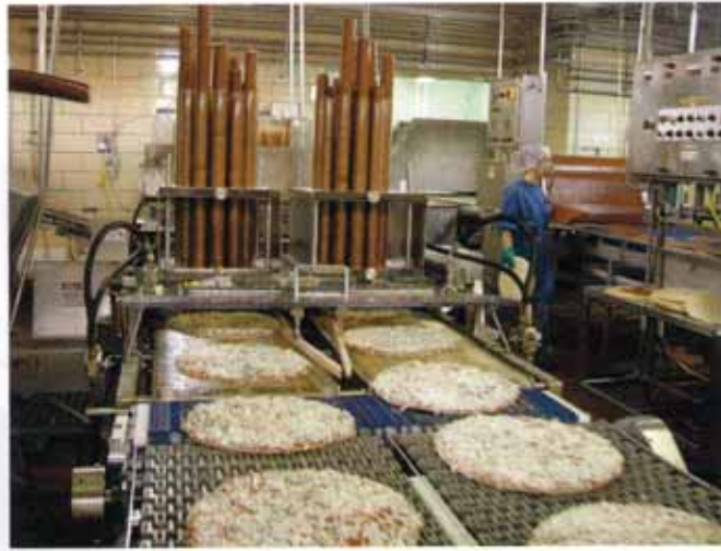
▲ After being topped with cheese, these 12.5-in. pizzas are ready for topping with pepperoni from this automatic slicer.
